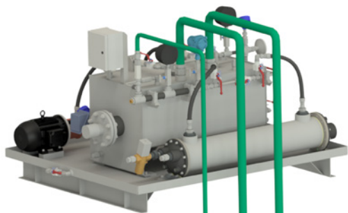
Figure 24: Head shaft bearing lubrication system
